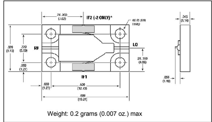
\*For the base model, only the IF1 port is connected.
