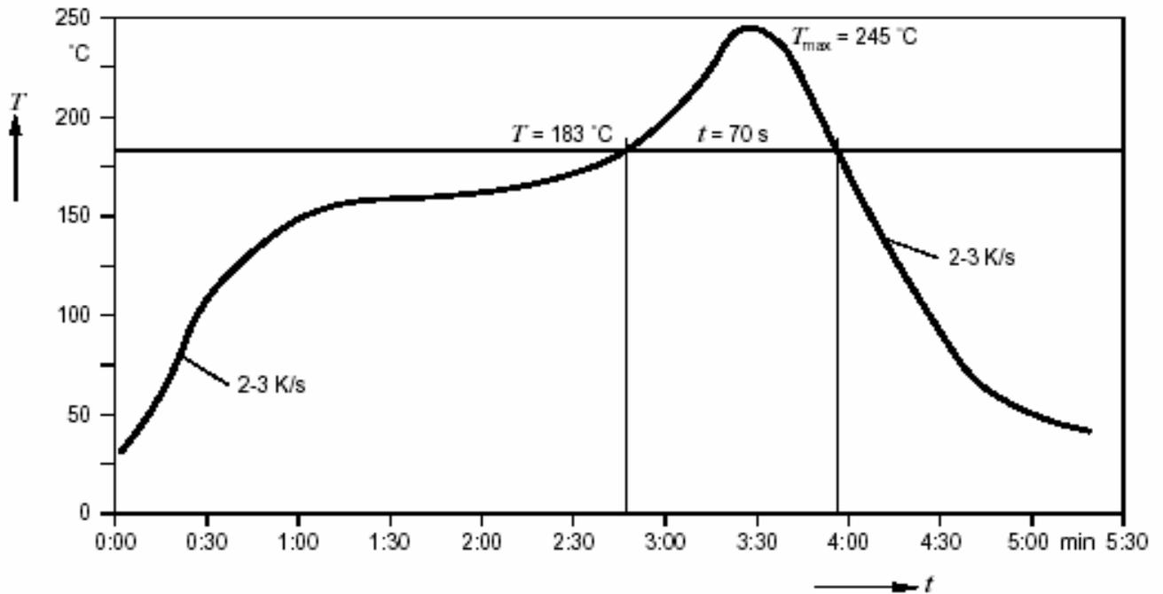
● Suggest Sn/Pb IR Reflow Soldering Profile Condition:
