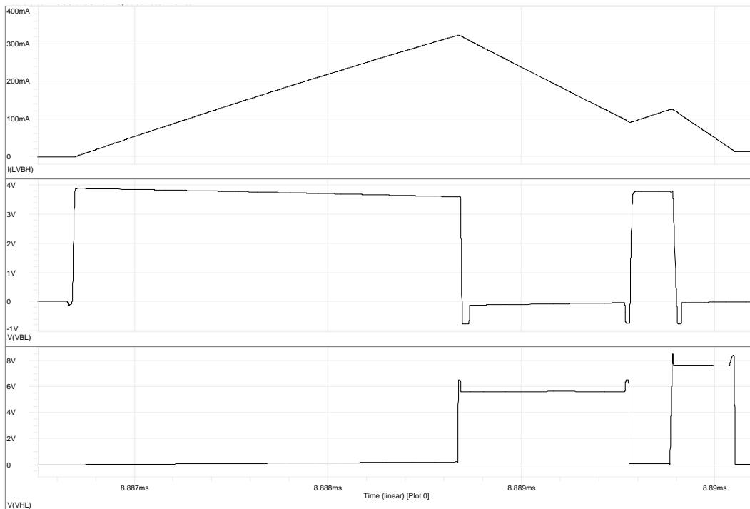
Figure 2: Converter current/voltage characteristics (VB = 4 V)
