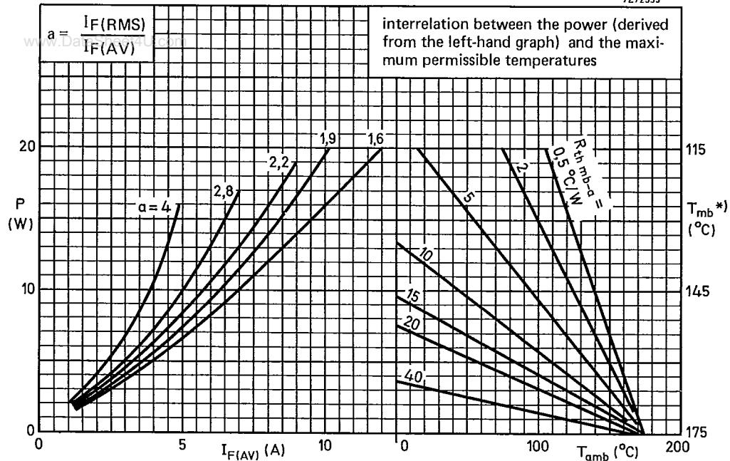
\*)  $T_{mb}$ -scale is for comparison purposes only and is correct only for  $R_{th\ mb-a} \leq 22\ ^{\circ}\text{C}/\text{W}$
