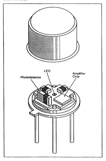
Photodetector technology is finding increasing use in liquid and gas monitoring systems. The existance and level of pollutants can be determined by their effect on the transmission of light through the medium concerned.
