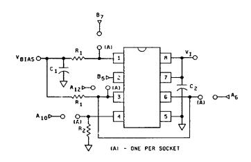
NOTES: 1.  $R_1 = 625$  ohm, 1/4 watt, 5 percent. 2.  $R_2 = 1$  K ohm, 1/4 watt, 5 percent. 3.  $C_1 = 1.0 \, \mu\text{F}$ , 50 volt, X7R (1 per socket). 4.  $C_2 = 0.1 \, \mu\text{F}$ , 50 volt, X7R (1 per socket). 5.  $I_{\text{CCA}} = 23$  mA per unit (350 units maximum per board). 6. Pins 1, 3, 4, and 6 must go to an eyelet that can be jumpered to the designated
