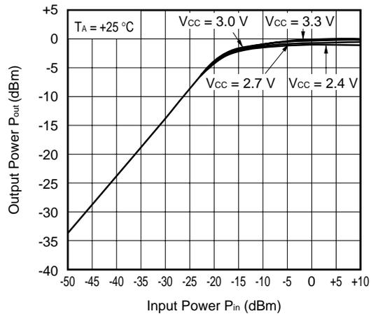
Output Power of Each Tone and 3rd Order Intermodulation Distortion vs. Input Power of Each Tone
