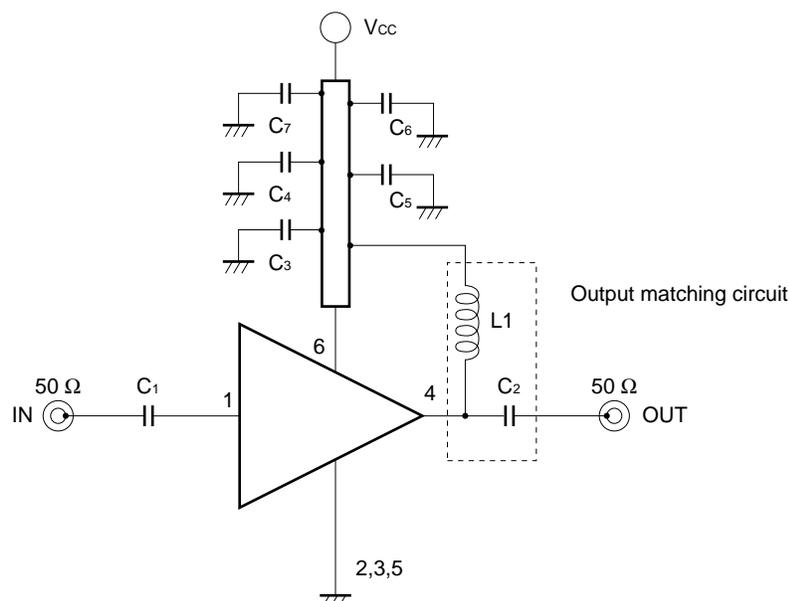
This test circuit is used in an NEC measurement jig. Multiple bypass capacitors are used in the V<sub>CC</sub> line due to the board pattern design of the NEC jig. The number of bypass capacitors should be reduced by optimizing the circuit board pattern when performing an actual application.
