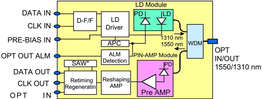
SAW: Surface Acoustic Wave Filter
