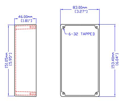
NOTE; FOR DETAIL DIMENSIONING REFER TO DRAWING # 1590F
