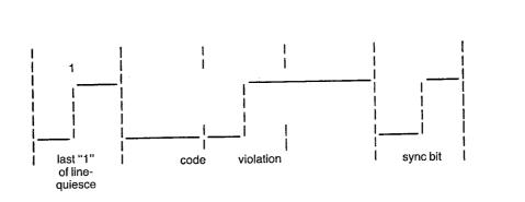
The Code Violation pattern is a bit sequence containing no mid-bit time level transition in two of its three bit cells. It is a unique pattern that violates the encoding rules and indicates the start of valid data.
