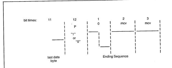
The Mini Code Violation (MCV) pattern is a bit sequence containing no mid-bit time level transition in either of its bit cells. It is a unique code that violates the encoding rules and indicates the end of valid transmit data.
