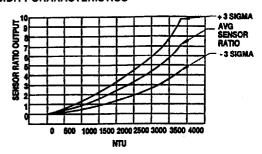
This graph is based on testing using formazin as the medium at room temperature. Characteristics may change when sensor is subjected to media other than formazin.
