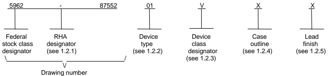
1.2.1 RHA designator. Device classes Q and V RHA marked devices meet the MIL-PRF-38535 specified RHA levels and are marked with the appropriate RHA designator. Device class M RHA marked devices meet the MIL-PRF-38535, appendix A specified RHA levels and are marked with the appropriate RHA designator. A dash (-) indicates a non-RHA device.
