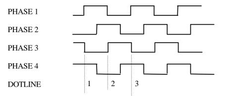
There are four different positions for the stepper motor. The driving is bipolar and can be achieved with circuits like Rohm BA6845FS, Sanyo LB1836 or LB1838 or Hitachi HA13421. Please refer to the IC's data sheet for further information. It is recommended not to exceed 0.2v like voltage drop in the stepper motor driver circuit.
