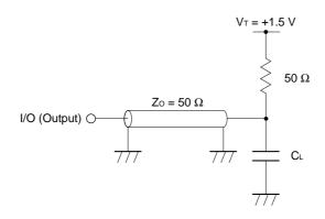
Remark CL includes capacitances of the probe and jig, and stray capacitances.
