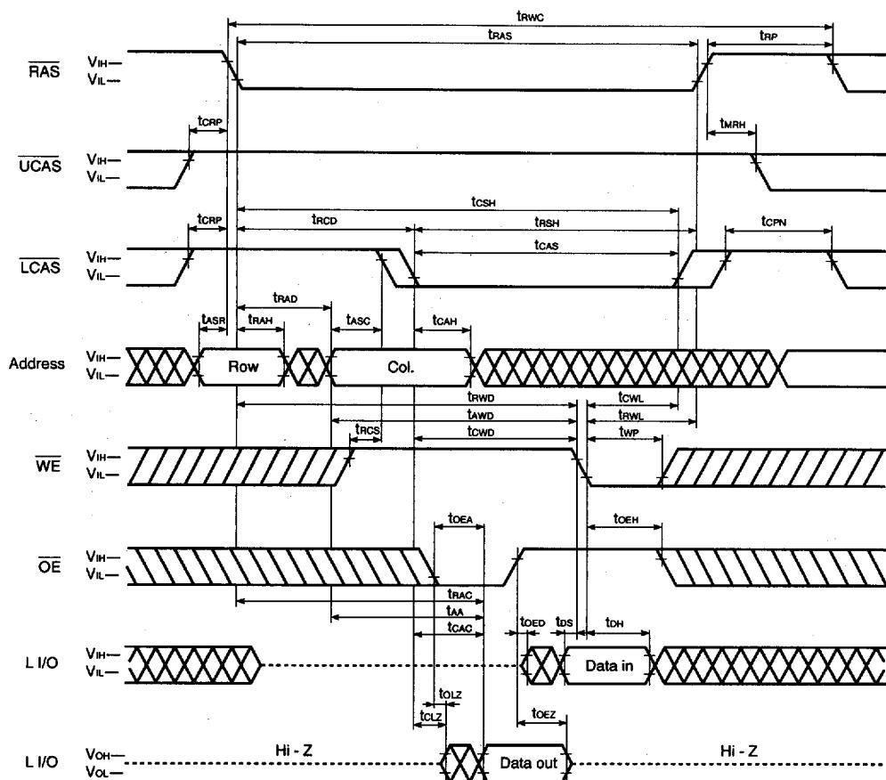
**Remark** In this cycle, the input data to Upper I/O is ineffective. The data out of that remains Hi-Z.
