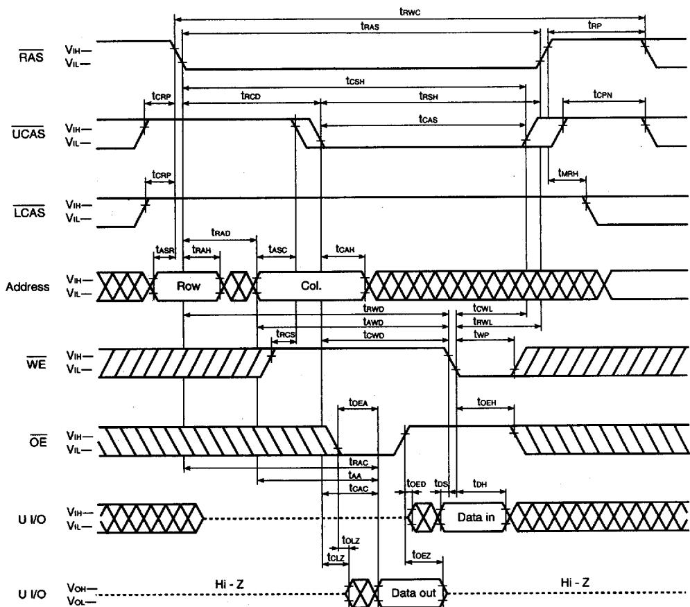
**Remark** In this cycle, the input data to Lower I/O is ineffective. The data out of that remains Hi-Z.
