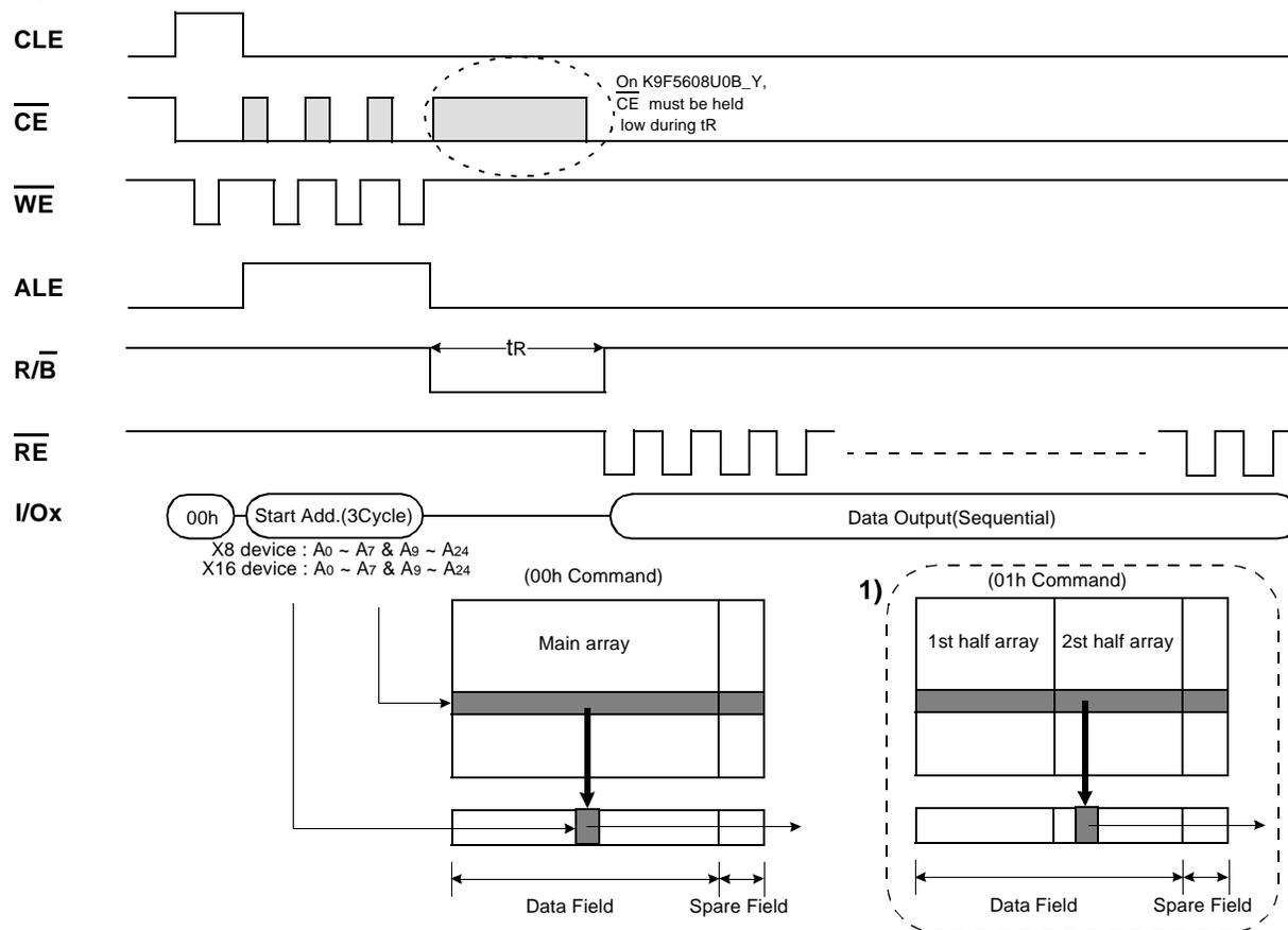
NOTE: 1) After data access on 2nd half array by 01h command, the start pointer is automatically moved to 1st half array (00h) at next cycle. 01h command is only available on X8 device(K9F5608X0B).
