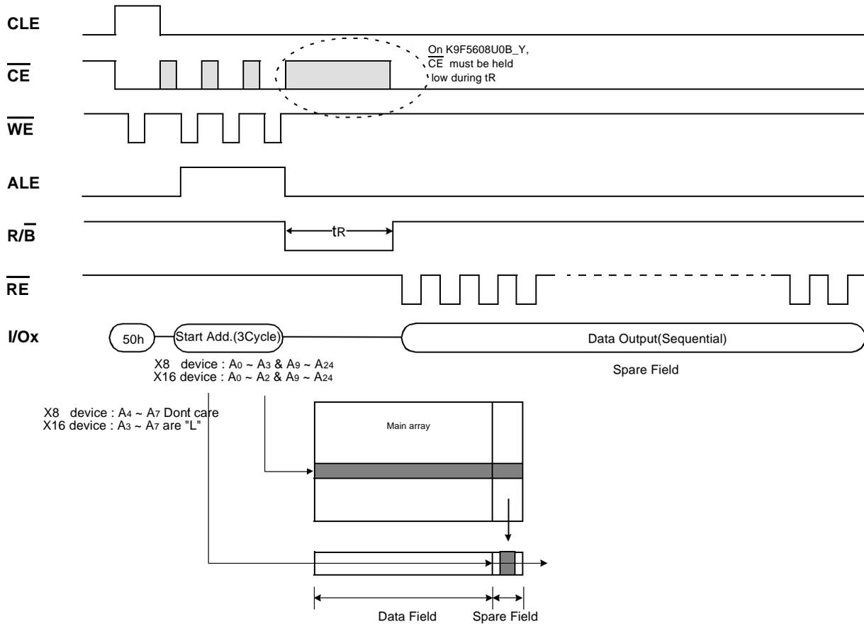
**Figure 7-1. Sequential Row Read1 Operation (K9F5608U0B-Y only)**
