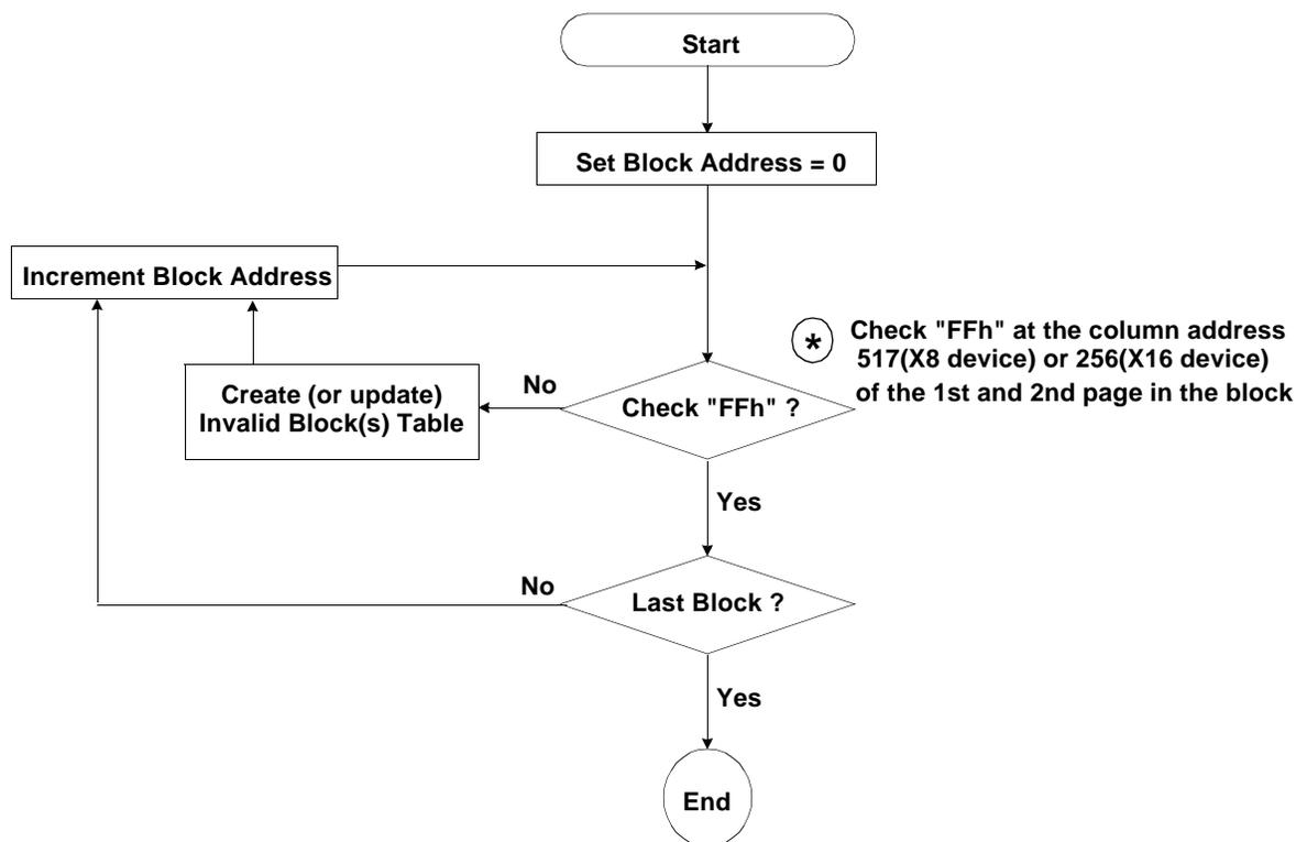
Figure 3. Flow chart to create invalid block table.
