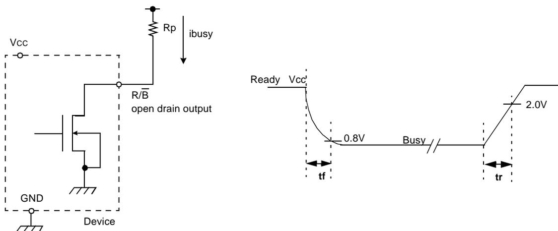
**Fig 14 Rp vs tr ,tf & Rp vs ibusy**
