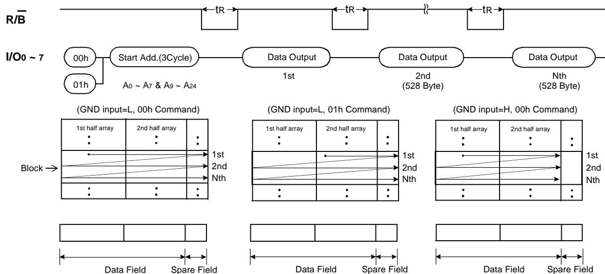
Figure 8-1. Sequential Row Read2 Operation (GND Input=Fixed Low) (K9F5608U0B-Y only)
