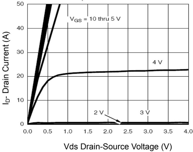
Figure 1 Output Characteristics
