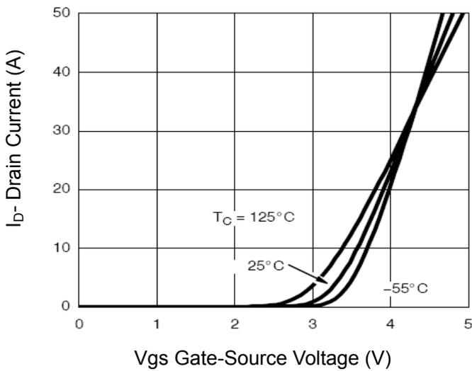
Figure 2 Transfer Characteristics
