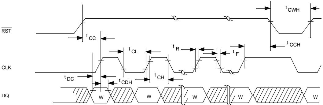
**3-WIRE READ DATA TIMING DIAGRAM Figure 20**
