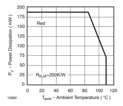
Figure 1. Power Dissipation vs. Ambient Temperature
