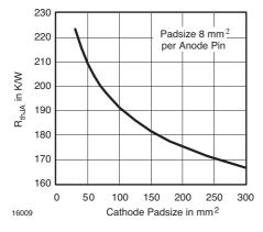
Figure 6. Thermal Resistance Junction Ambient vs. Cathode Padsize
