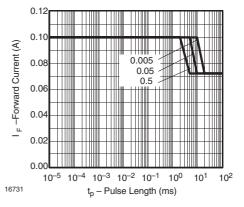
Figure 3. Forward Current vs. Pulse Length
