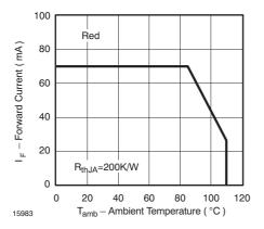
Figure 2. Forward Current vs. Ambient Temperature
