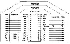
Note: JEDEC standard pinouts for AT27C011 and AT27C128 are shown for comparison only.
