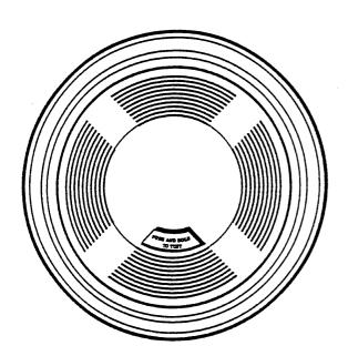
This Dicon Linkable Photoelectric Smoke and Fire Alarm is a 9 volt battery powered device utilising a sensing technology that "sees" smoke. This makes the unit ideal for detecting slow smouldering fires. The alarm can be linked to as many as 11 other alarms. This extends security economically over a large area. Pressing and holding the test button confirms the link is operating.
