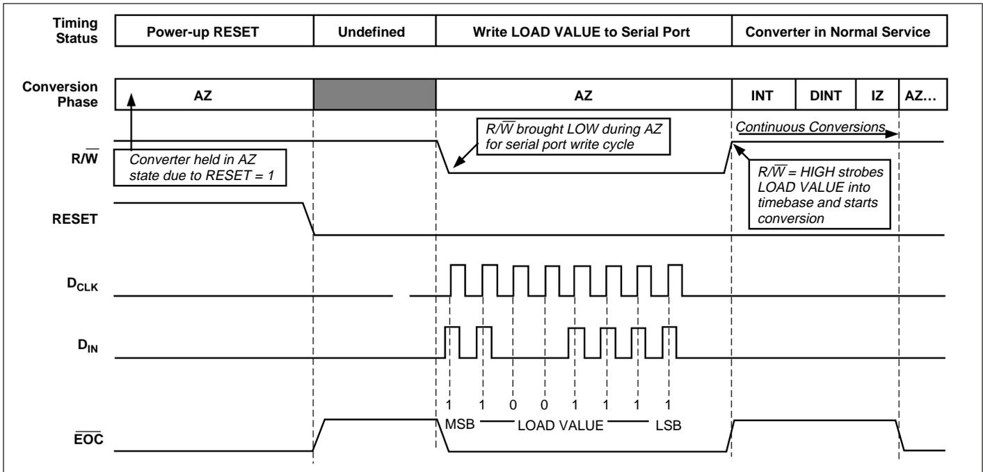
Figure 4. TC530/534 Initialization and Load Value Write Cycle
