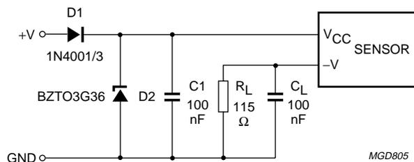
Fig.8 Test/application circuit for the KMI20/2.
