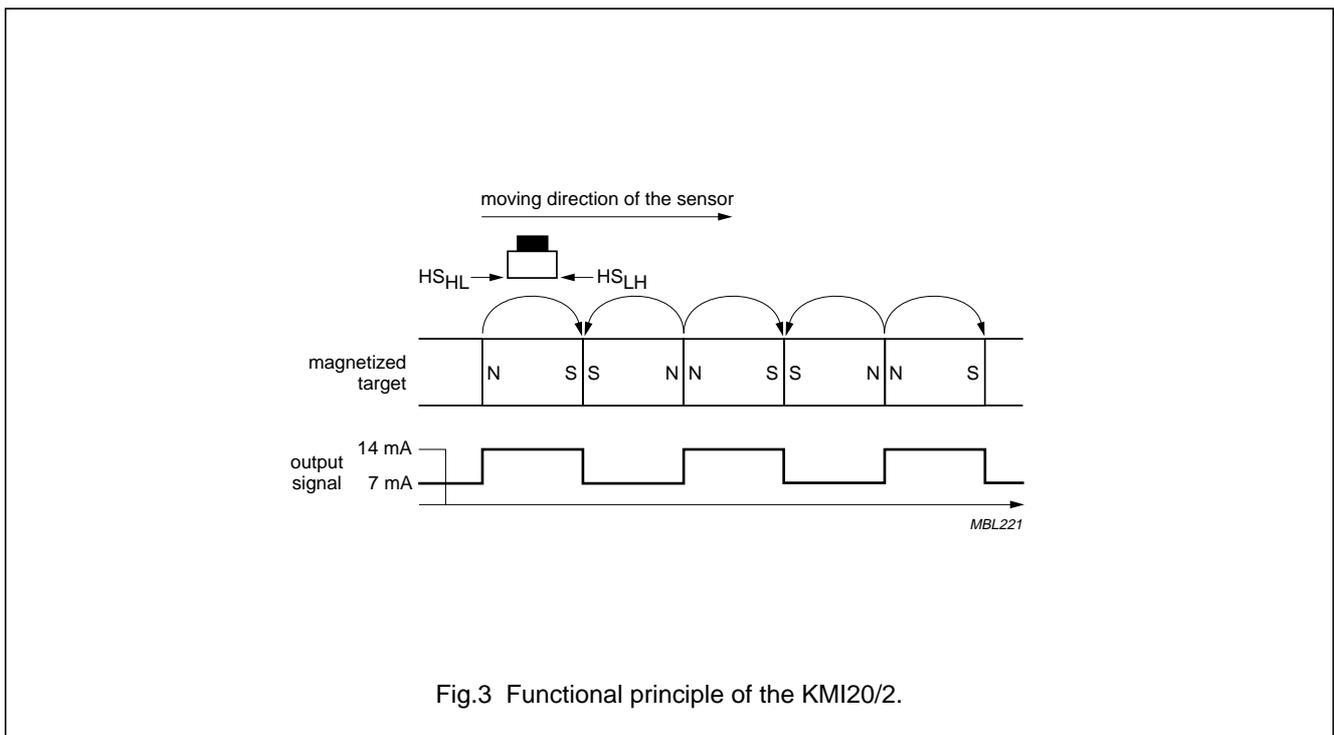
Rotational speed sensor for extended air gap application
