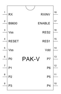
**WARNING:** The PAK V is a static-sensitive, CMOS device. Observe static precautions when handling. Operating the device without both Vss pins grounded or with RES1 or RES2 disconnected may damage the chip.
