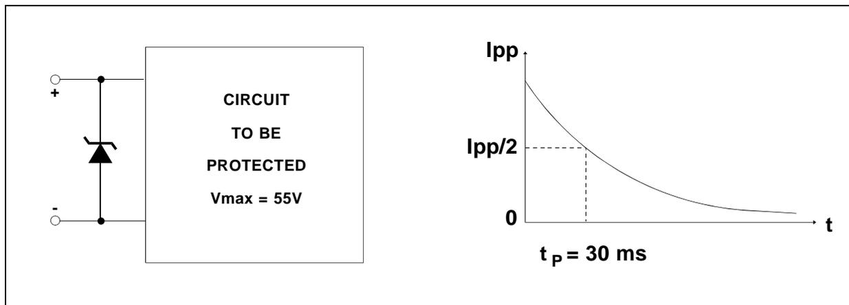
$V_{RM} > V_{CC} = 30V$  and  $V_{CL} max < 55V$  with a maximum ambient temperature of  $50^{\circ}C$ .
