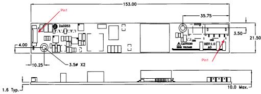
Note: Please use plastic screw in case of a non-insulating mounting base!
