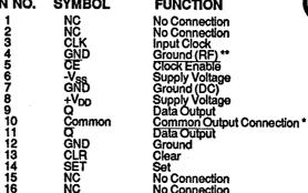
No Connection \* Connect the common output connection to ground for ECL level output.
