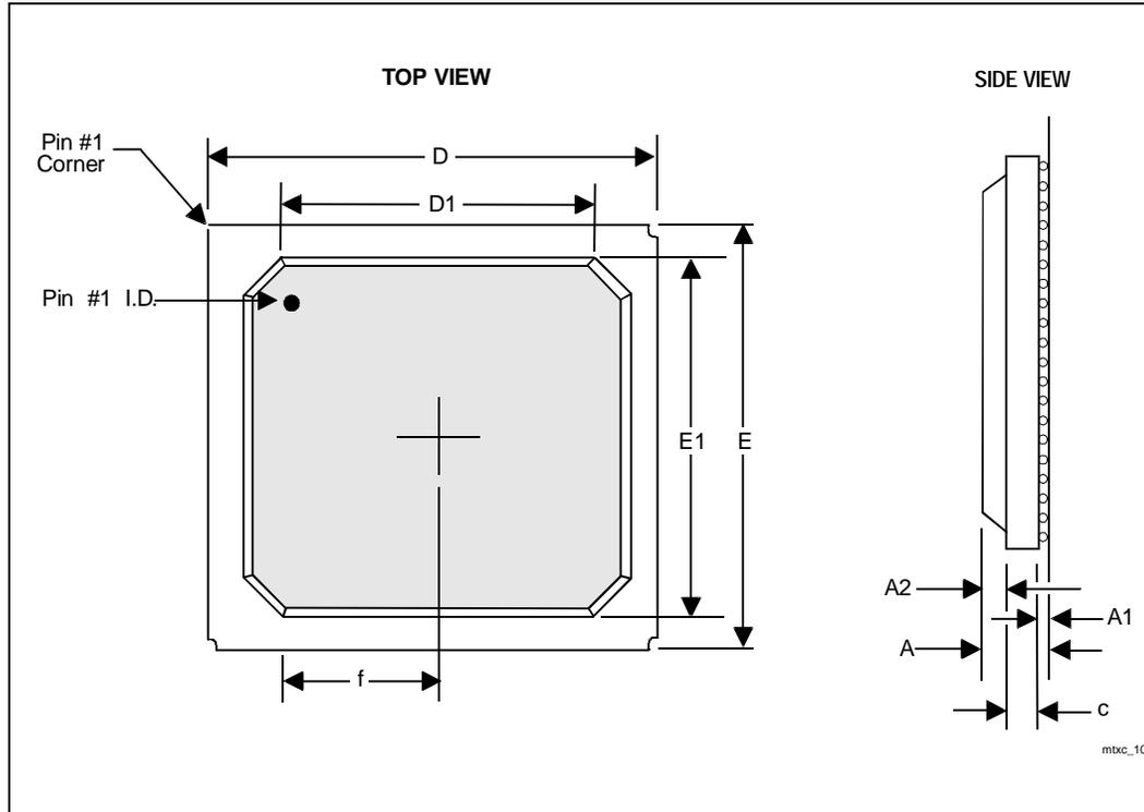
Figure 13. MTXC 324-pin Ball Grid Array (BGA)
