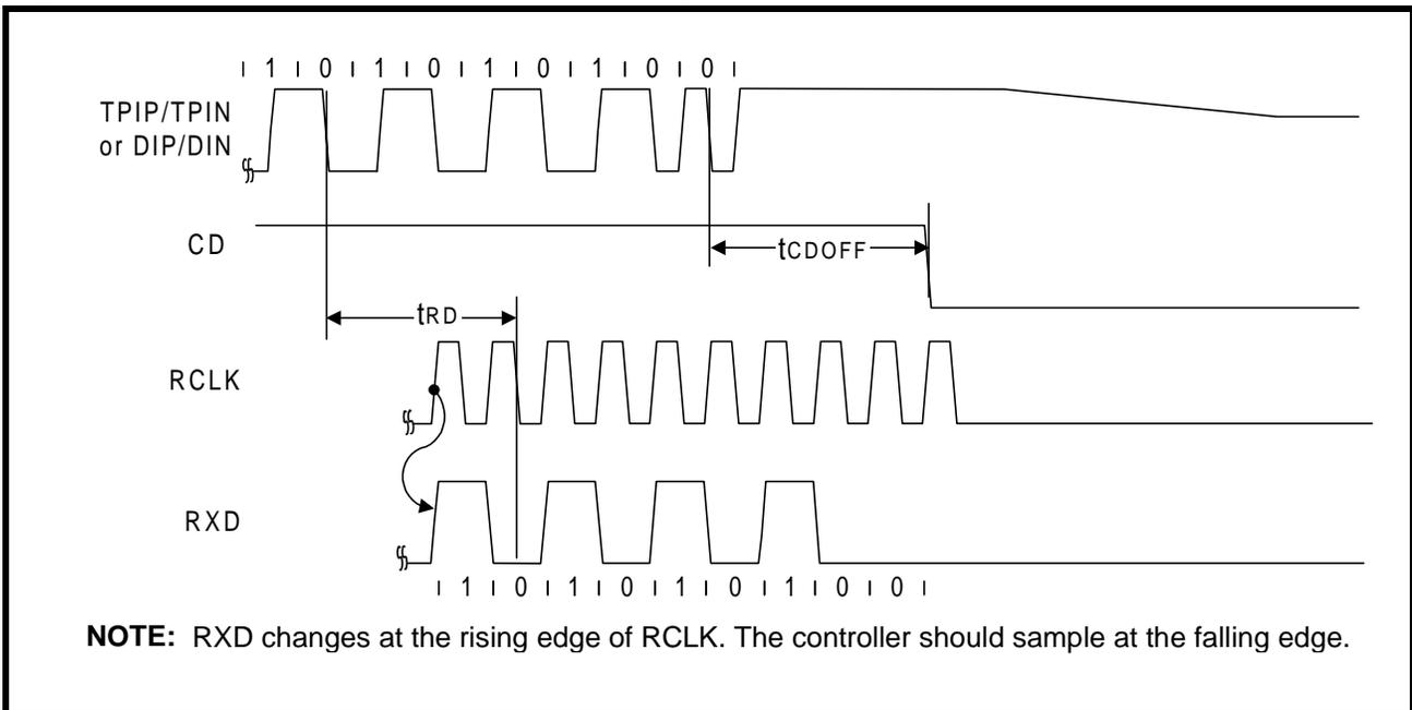
Figure 23: Mode 2 Transmit Timing
