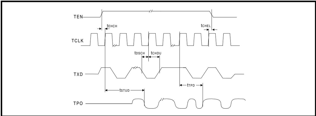
Figure 36: Mode 4 Collision Detect Timing
