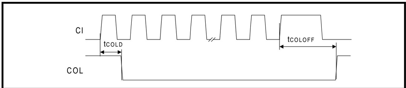
Figure 31: Mode 3 COL/SQE Output Timing
