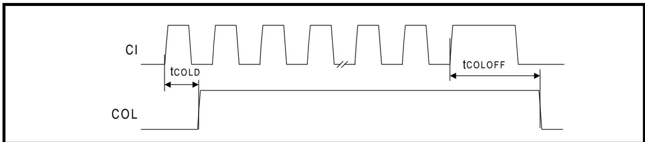
**Figure 43: Mode 5 COL/SQE Output Timing**
