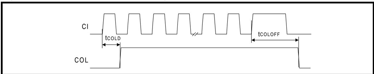
Figure 37: Mode 4 COL/SQE Output Timing
