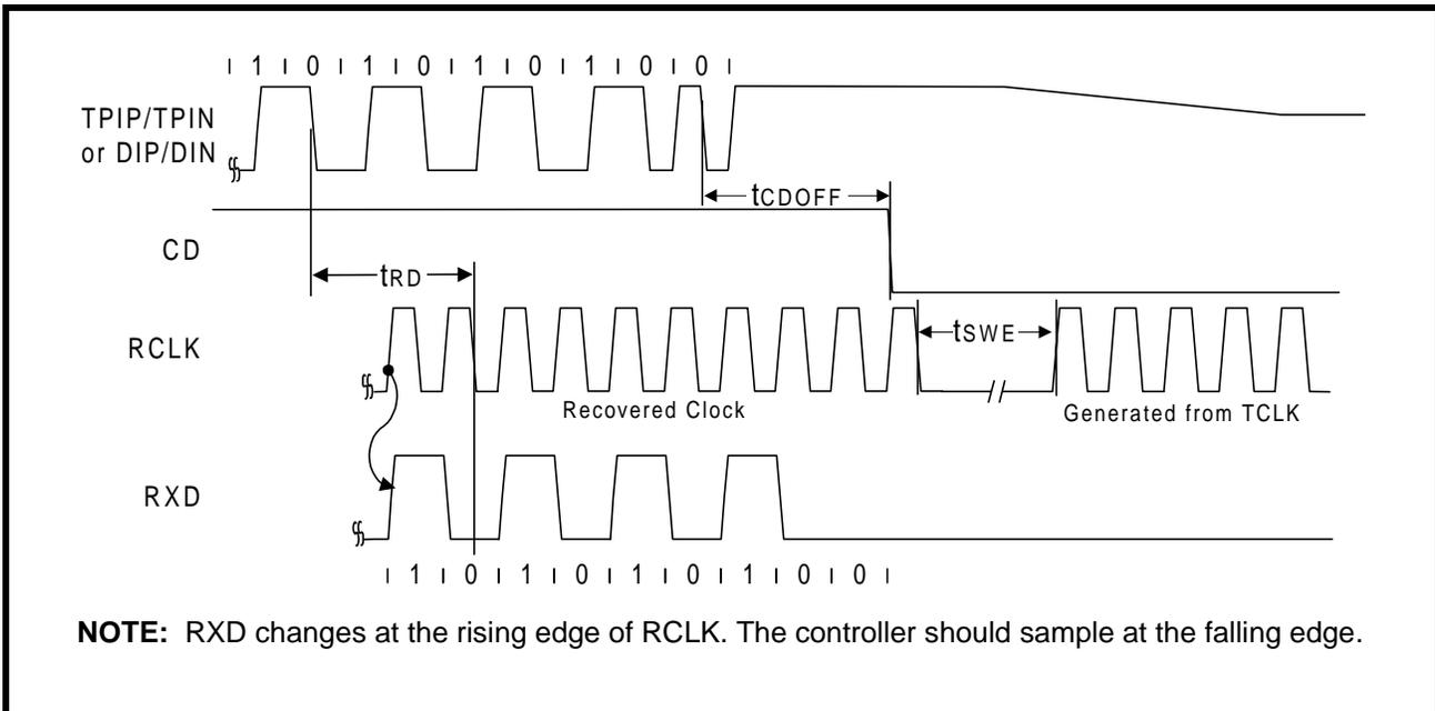
Figure 29: Mode 3 Transmit Timing
