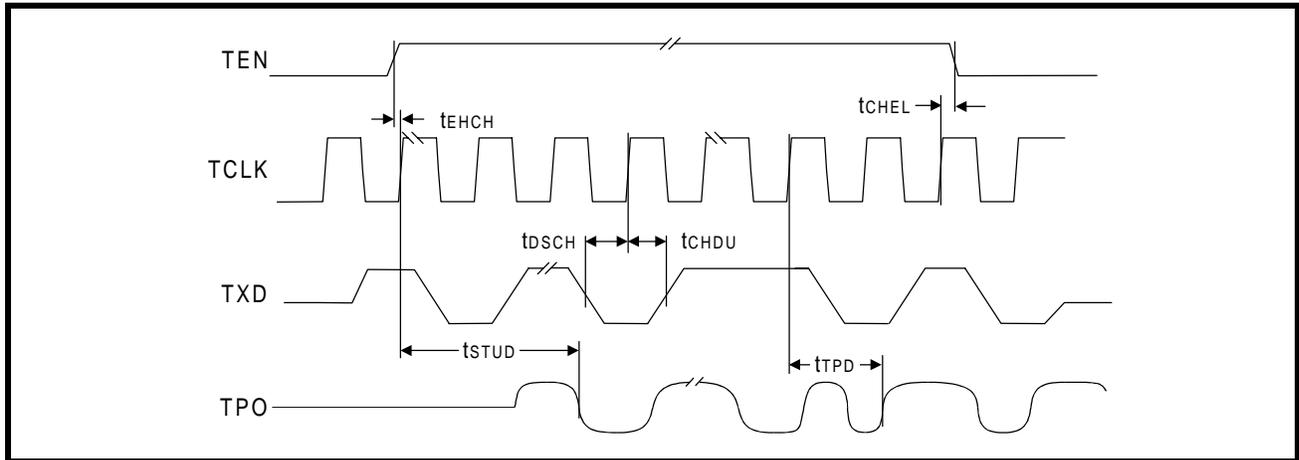
**Figure 42: Mode 5 Collision Detect Timing**
