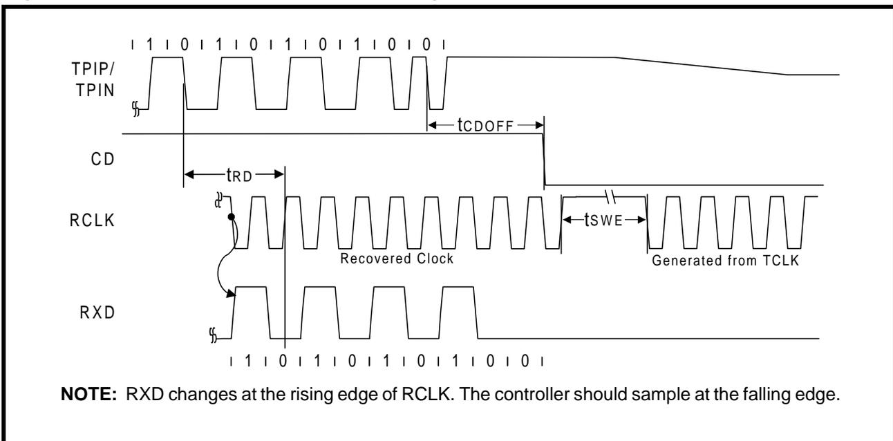
**Figure 41: Mode 5 Transmit Timing**
