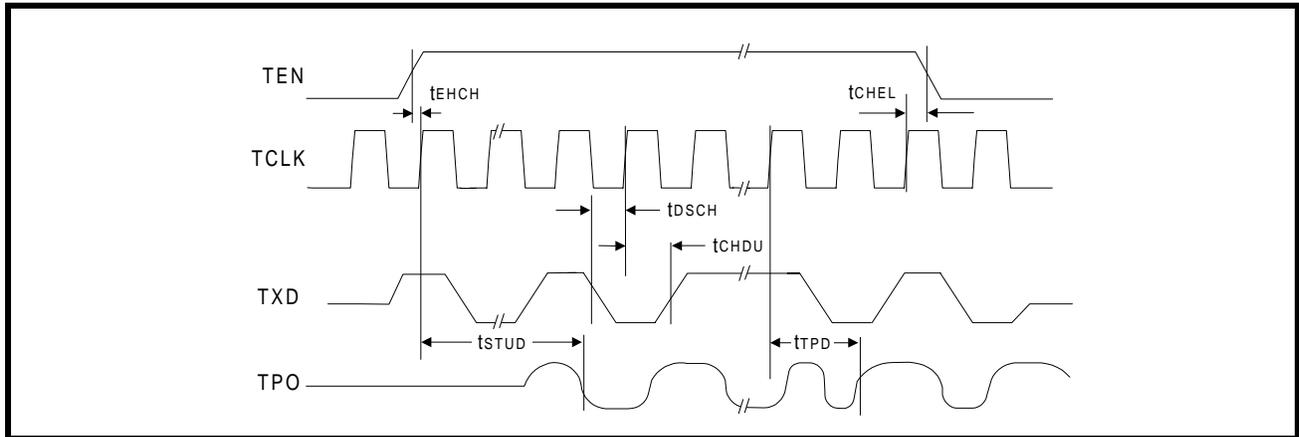
Figure 18: Mode 1 Collision Detect Timing
