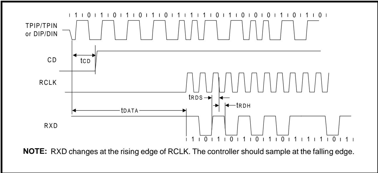
Figure 22: Mode 2 RCLK/End-of-Frame Timing
