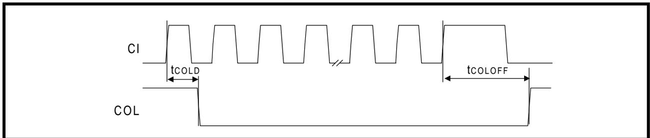
Figure 25: Mode 2 COL/SQE Output Timing
