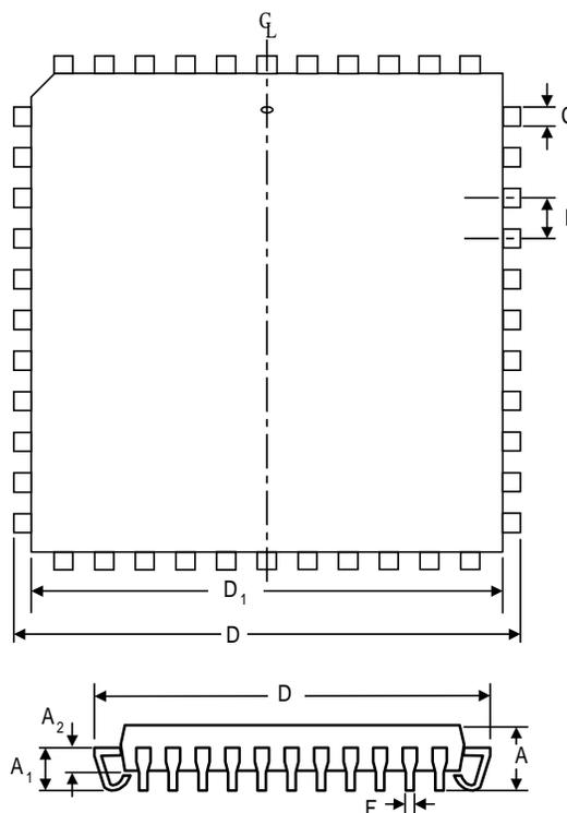
Figure 46: 64-Pin LQFP Package Specifications
