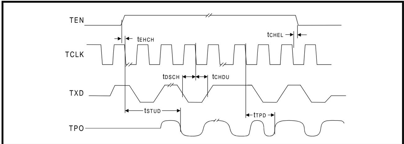
Figure 30: Mode 3 Collision Detect Timing
