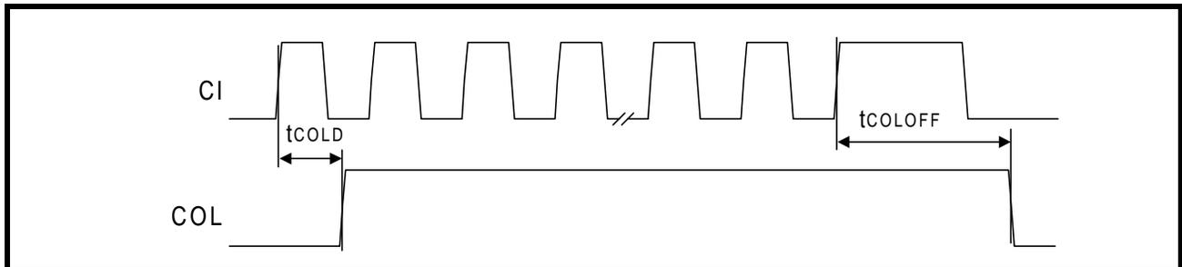
Figure 19: Mode 1 COL/SQE Output Timing/CI Output Timing
