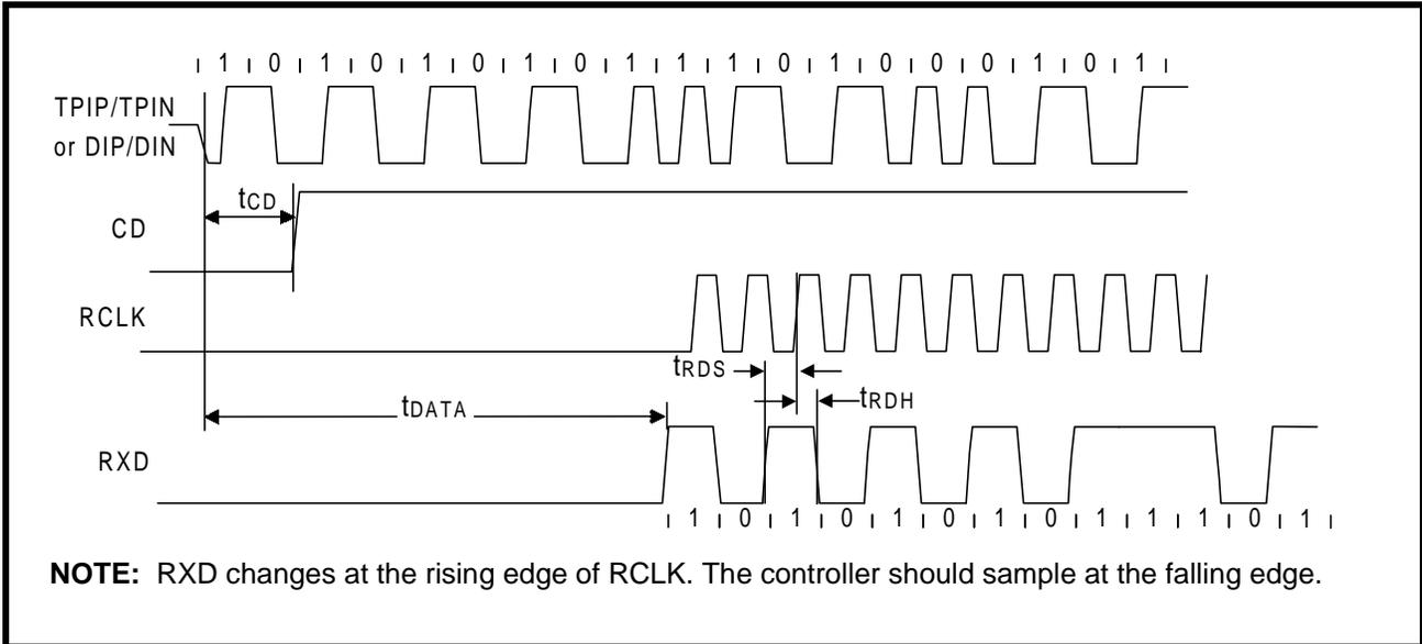
**Figure 34: Mode 4 RCLK/End-of-Frame Timing**
