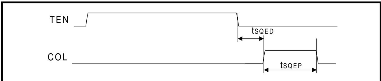
Figure 38: Mode 4 Loopback Timing
