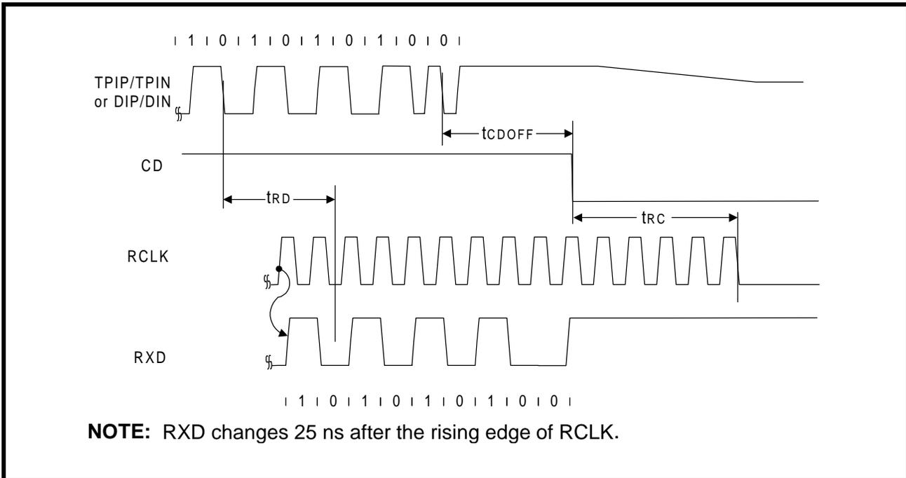
Figure 17: Mode 1 Transmit Timing
