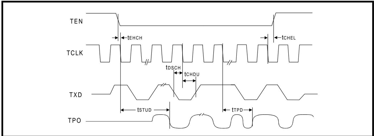
Figure 24: Mode 2 Collision Detect Timing
