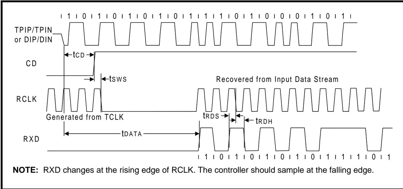
Figure 28: Mode 3 RCLK/End-of-Frame Timing
