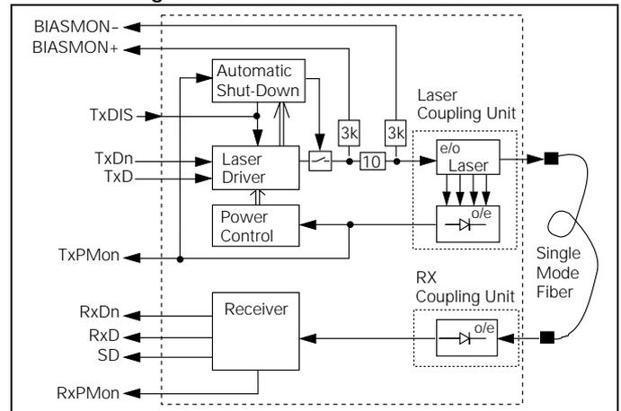
The receiver component converts the optical serial data into PECL compatible electrical data (RxD and RxDn). The Signal Detect (SD, active high) shows whether an optical signal is present<sup>(1)</sup>. If no optical input signal is present the receiver data outputs are switched to static low level (RxD=0, RxDn=high).
