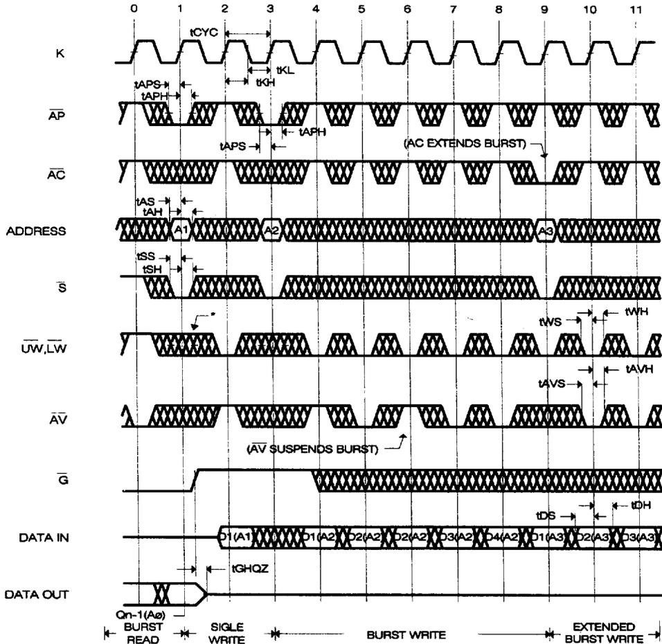
\* When  $\overline{AP}$  initiates the burst sequence, the  $\overline{W}$  control input is ignored for the first cycle, The  $\overline{W}$  and DATA IN should be asserted and registered in the subsequent cycle.
