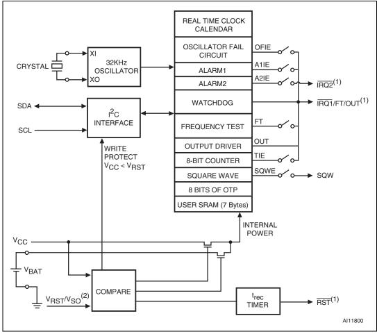
Figure 8. M41T83 block diagram
