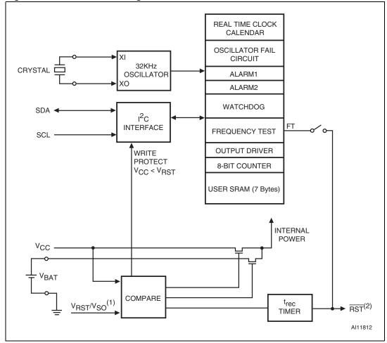
Figure 6. M41T82 block diagram
