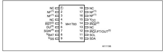
1. NF pins must be tied to  $V_{SS}$ . Pins 2 and 3, and 16 and 17 are internally shorted together.
