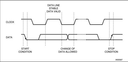
Figure 10. Serial bus data transfer sequence
