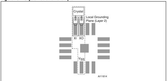
Figure 20. Crystal isolation example
