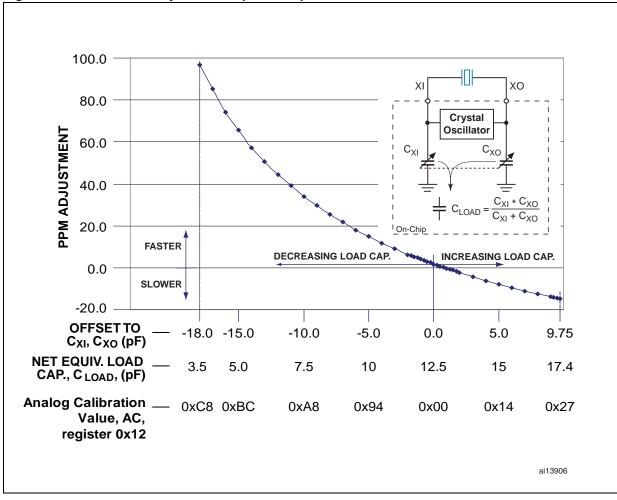
Figure 18. Clock accuracy vs. on-chip load capacitance
