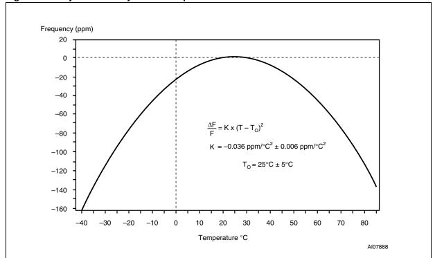
Figure 17. Crystal accuracy across temperature
