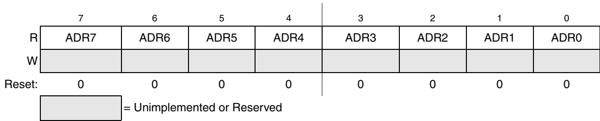
Figure 14-7. Data Result Low Register (ADC1RL)
