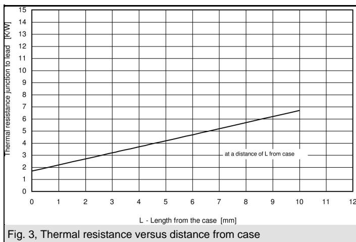
Fig. 3, Thermal resistance versus distance from case
