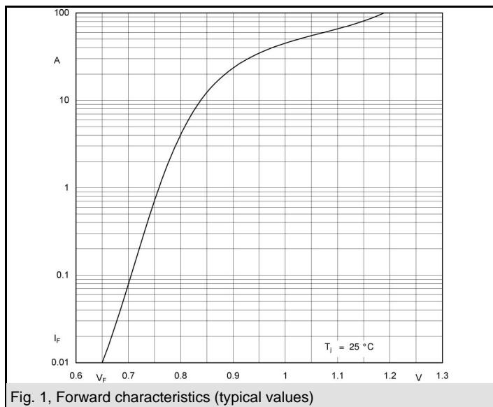
Fig. 1, Forward characteristics (typical values)
