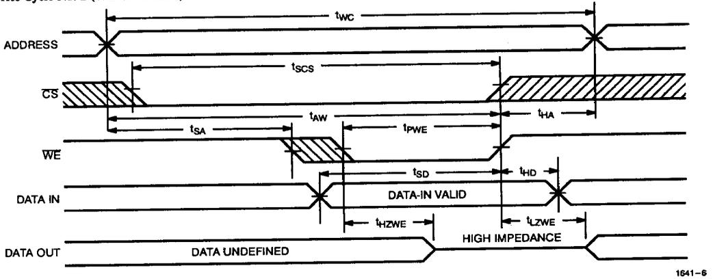
Write Cycle No. 2 (CS Controlled)<sup>[7, 10]</sup>
