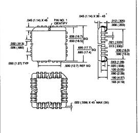
32L, 32 Pad, Non-Windowed, Ceramic Leadless Chip Carrier (LCC) Dimensions in Inches and (Millimeters)
