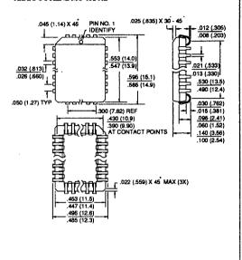
44J, 44 Lead, Plastic J-Leaded Chip Carrier (PLCC) Dimensions in Inches and (Millimeters) JEDEC OUTLINE MO-047 AC
