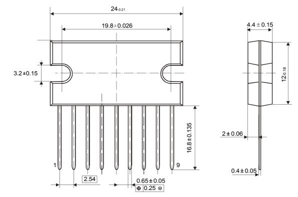
• 9-Pin Plastic Power Single-in-Line (SIL-9MPF, SOT 131-2)
