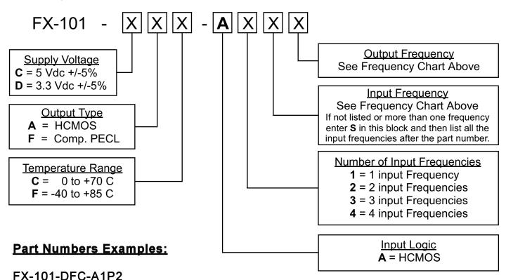
FX-101-DFC-A4S2 - 8 kHz, 1.544 MHz, 2.048 MHz, 19.44 MHz
