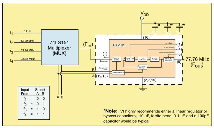
All components outside the dotted line box are user supplied components and/or connections. This is just one possible configuration of the FX-101. For additional information about your specific needs please contact our Factory.
