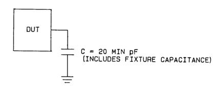
FIGURE 4. Waveforms and test circuit.
