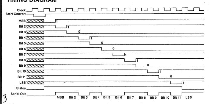
Data may be sent in serial format and converted to parallel as shown. This process can reduce the number of transmission lines from 14 to 3 for a 12-bit A/D converter.
