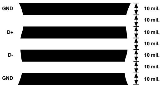
Figure 12. Arrangement of Signal Tracks
