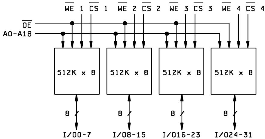
FIGURE 6. Block diagram, case outlines M, U, X, Y, Z and 4.
