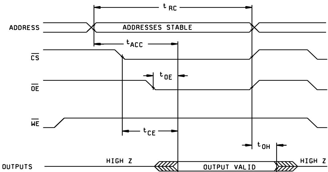
FIGURE 4. Read cycle timing diagram.
