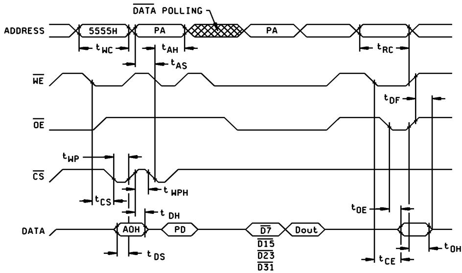
FIGURE 5. Write/Erase/Program operations, WE controlled.
