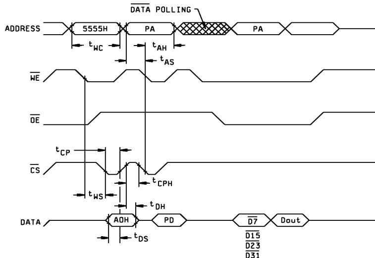
FIGURE 5. Write/Erase/Program operations, CS controlled.
