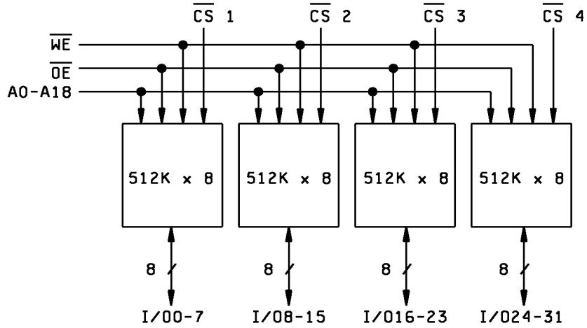
FIGURE 6. Block diagram, case outlines N and T.
