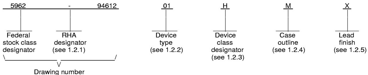
1.2.1 Radiation hardness assurance (RHA) designator. Device classes H and K RHA marked devices shall meet the MIL-PRF-38534 specified RHA levels and shall be marked with the appropriate RHA designator. A dash (-) indicates a non-RHA device.
