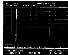
Figure 12. Spectral Response of Digitally Constructed Sine Wave
