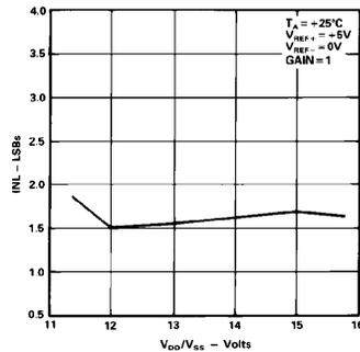
Figure 13. Typical Linearity vs.  $V_{DD}/V_{SS}$
