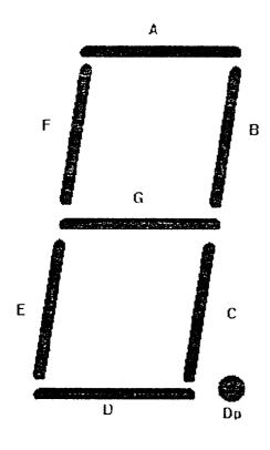
Example 6 - to send the character S to digit 5. First calculate which segments are on and which are off.
