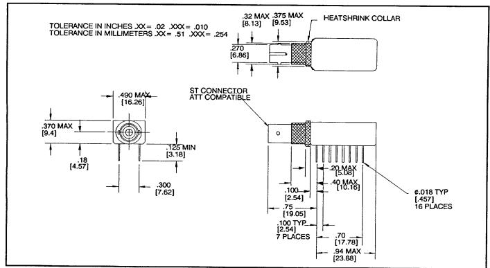
The metal housing is conductive and should be prevented from contacting circuit board traces or the sleeves of low profile screw machine
