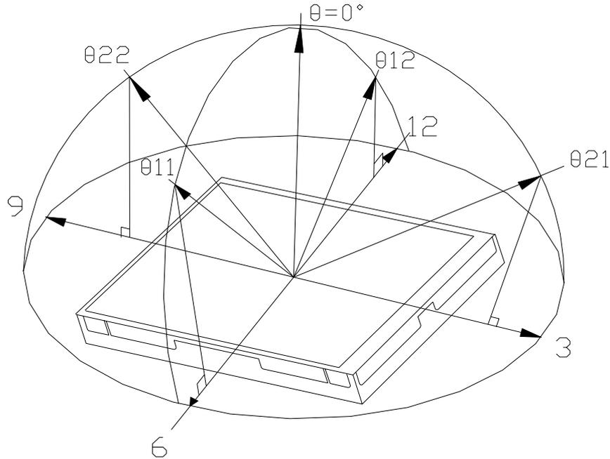
Note 10-2 :  $CR = \frac{\text{Luminance when Testing point is White}}{\text{Luminance when Testing point is Black}}$
