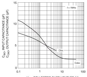
V<sub>CB</sub>, COLLECTOR-BASE VOLTAGE (V) Fig. 2, Input and Output Capacitance vs. Collector-Base Voltage
