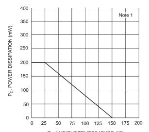
T<sub>A</sub>, AMBIENT TEMPERATURE (°C) Fig. 1, Max Power Dissipation vs Ambient Temperature
