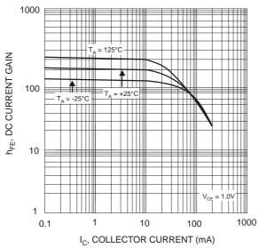
I<sub>C</sub>, COLLECTOR CURRENT (mA) Fig. 3, Typical DC Current Gain vs Collector Current
