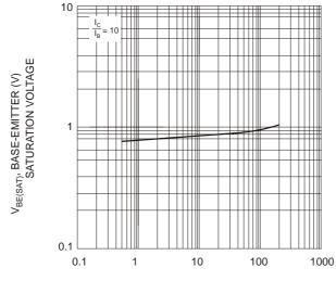
I<sub>C</sub>, COLLECTOR CURRENT (mA) Fig. 5, Typical Base-Emitter Saturation Voltage vs. Collector Current
