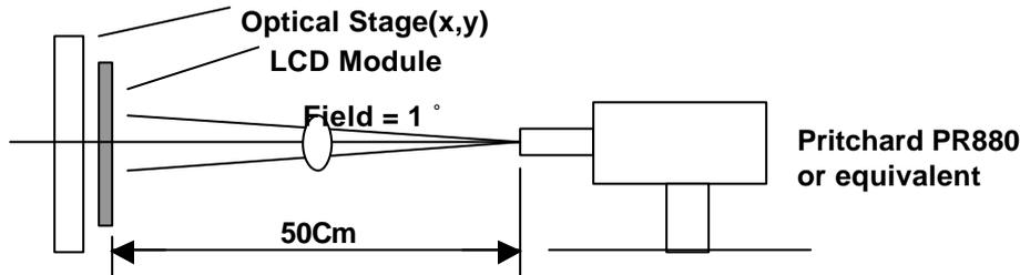
[Figure 9] Optical characteristic measurement equipment and method
