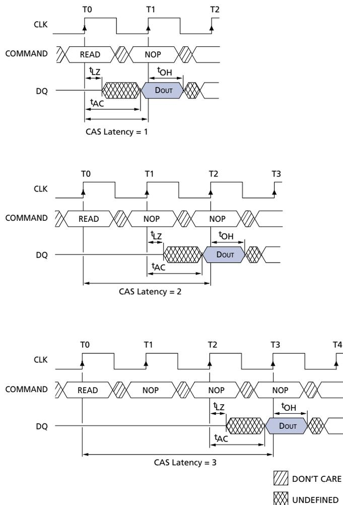
element  $n + 3$  is either the last of a burst of four or the last desired of a longer burst. This 256Mb SDRAM uses a pipelined architecture and therefore does not require the  $2n$  rule associated with a prefetch architecture. A READ command can be initiated on any clock cycle
