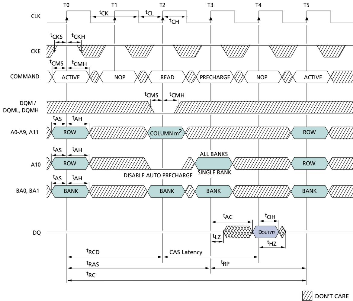
**NOTE:** 1. For this example, the burst length = 1, the CAS latency = 2, and the READ burst is followed by a "manual" PRECHARGE.
