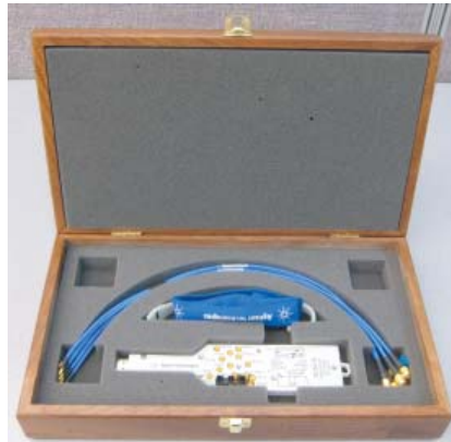
Figure 18. The Agilent W2641A DisplayPort test point adapter fixture
